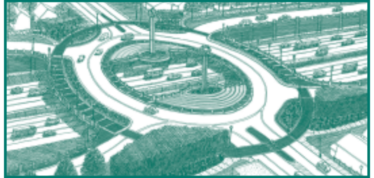
An “elipsabout” at the proposed 38th Street exit would calm the flow of traffic moving on and off the freeway.
